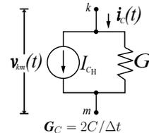
$G_C = 2C/\Delta t$ $i_C(t) = I_{C_H}(t - \Delta t) + G_C(v_C(t))$ $I_{C_H}(t - \Delta t) = -i_C(t - \Delta t) - G_C(v_C(t - \Delta t))$                                                                              |
