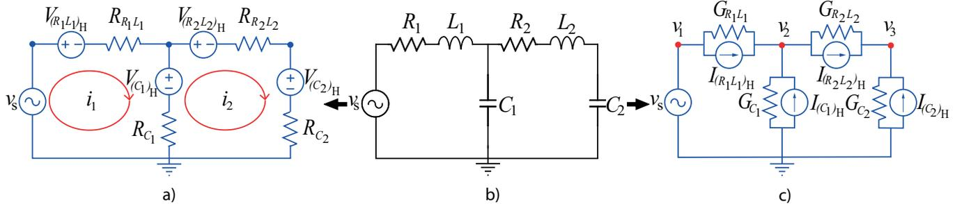
Fig. 2: Electric network with  $RL$  branches: a) Equivalent diagram by applying  $CCA_{Th}$ , b) Electric network, c) Equivalent diagram by applying  $CCA_N$ .
