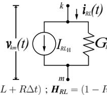
$G_{RL} = \Delta t/(2L + R\Delta t) ; H_{RL} = (1 - RG_L)/(1 + RG_L)$ $i_{RL}(t) = I_{RL_H}(t - \Delta t) + G_{RL}(v_{km}(t))$ $I_{RL_H}(t - \Delta t) = H_{RL}(i_{RL}(t - \Delta t)) + G_{RL}(v_{km}(t - \Delta t))$ |
