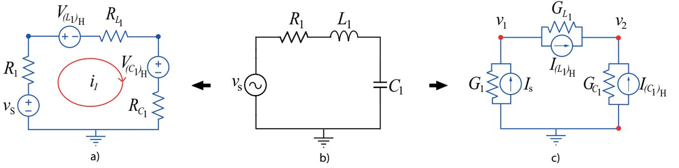
Fig. 1: Series  $RLC$  electric circuit: a) Equivalent circuit by using  $CCA_{Th}$ , b) Electric circuit, c) Equivalent circuit by using  $CCA_N$ .
