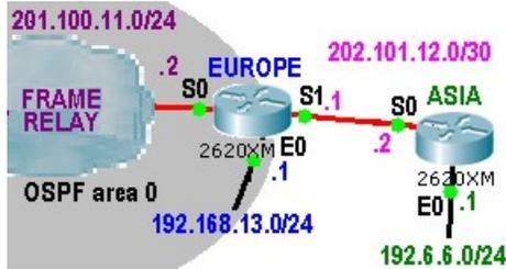
It has created an Internetwork where a router EUROPE and a router called ASIA are connected by serial link using Point-to-Point.
