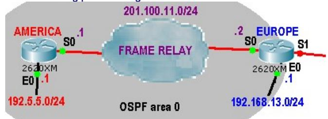
2. AMERICA and EUROPE are connected and configured already [3], the way to connect EUROPE and ASIA is the purpose of this paper, before already it has been configured and the way to configure the Point-to-Point Protocol between EUROPE router and ASIA router is very easy, only it does not forget the external route and OSPF single area.
