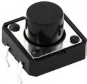
Switches, buttons, and contact sensors are used to detect physical contact between objects and are not just restricted to humans pushing buttons; bumpers on a robot can be equipped with momentary push buttons, and "whiskers" (just like a Pet) can be used to sense multiple distances. **Advantages:** very low cost, easy to integrate, reliable. **Disadvantages:** single distance measurement
